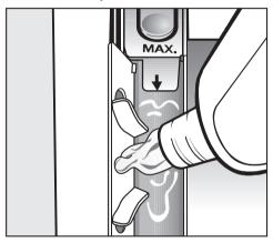
■ Add the fabric softener or liquid starch to compartment ⊗. Do not exceed the Max. level mark.
